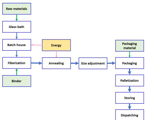
Fig.2: Scheme of the manufacturing process
